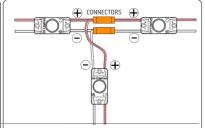
Modules may be connected in series or parrallel with connectors. Cap all unused wires. The strand of modules should not be looped to create a closed circuit.
