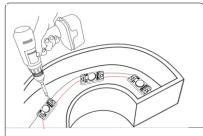
**3.** For firm fixing, use rivets or screws to secure LED module within the letter / box.
