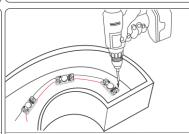
4. Drill the holes at the bottom or side of the letter / box for the wire connection to DC power supplies and grommet the hole for supply wire access.
