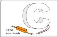
7. Run a wire from the power Supply to each channel letter and connect to the first LED module on the strip. Must be used with 12 V BaltLED Power Supplies.
