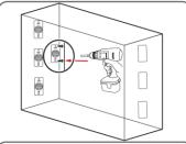
Screw the LED modules in the appropriate position in the light box.
