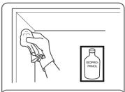
Clean the inside of the sign with a solvent (e.g.ethanol) to make sure it is free of dirt.
