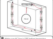
Make sure AC line is OFF before beginning power supply installation. Secure power supply to clean surface using screws. While connecting to modules do not mistade the polarity of (+) and (-).
