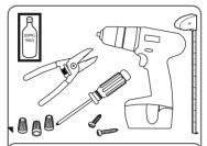
**1** Tools required. Wires, wire strippers, drill, screwdriver, screws, surface cleaner, therminal connectors anr measuring tape.
