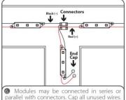
The strand of modules should not be looped to reate a closed circuit
