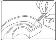
Using LED placement from step 1. remove tapes on the backside and stick LED modules into place.
