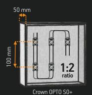
Thanks to the new optics we use in S+ series, the distance between centers of modules can be equal to the double depth of a signage application.
