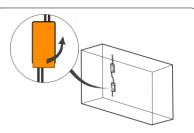
2. Remove protective layer from the backside of the module and stick LED modules into place.
