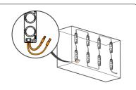
5. Cap all unused wires. The strand of modules should not be looped to create a closed circuit.
