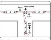
6. Modules may be connected in series of parallel with connectors. Cap all unused wires. The strand of modules should not be looped to create a closed circuit.
