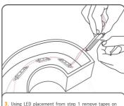
the backside and stick LED modules into place.
