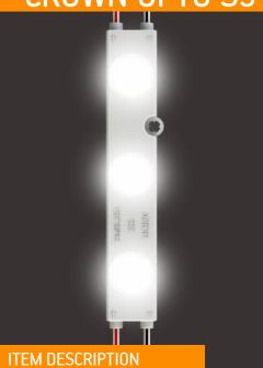
Crown OPTO STELLAR series modules are designed to illuminate bigger-depth letters and lightboxes. S3 module application is ranging from 120 to 200 mm in depth. These modules come with L70 100 000 h lifetime for 6500K and L70 50,000 h for other colours, granting 5 years warranty. Crown OPTO STELLAR — a great option for projects when economical, although a quality solution is needed.
