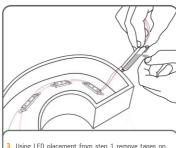
3. Using LED placement from step 1 remove tapes on the backside and stick LED modules into place.
