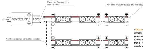
! 40 pcs - max number of modules in one chain when the power supplied from single end. ! String end voltage can't be less than 11V, do not exceed specified module string length
