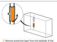
module and stick LED modules into place.
