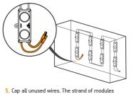
should not be looped to create a closed circuit.
