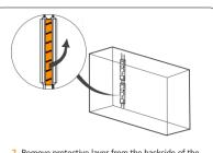
2. Remove protective layer from the backside of the module and stick LED modules into place.
