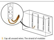
should not be looped to create a closed circuit.
