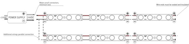
! 40 pcs - max number of modules in one chain when the power supplied from single end. ! String end voltage can't be less than 23V, do not exceed specified module string length
