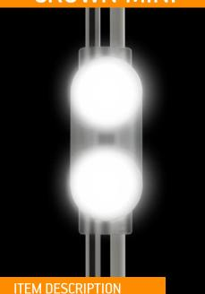
Crown MINI is best for the uniform illumination of shallow depth narrow channel letters. These modules are designed to fit in backlit and halo-lit applications with depths as low as 20 mm and widths as narrow as 8 mm. Great illumination uniformity can be achieved with 85 mm / 42 mm distance between modules and flexible silicone insulation wires allowing easy installation. A 5-year warranty with L70 for 50,000 hours is applied.
