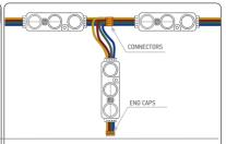
5. Modules may be connected in series or parrallel with connectors. Cap all unused wires. The strand of modules should not be looped to create a closed circuit.
