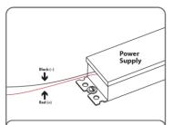
7. Run a wire from the power Supply to each channel letter and connect to the first LED module on the strip. Must be used with 12 V or 24 V BaltLED Power Supplies.
