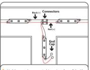
Modules may be connected in series of parallel with connectors. Cap all unused wires. The strand of modules should not be looped to create a closed circuit.
