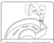
5. Drill the holes at the bottom or side of the letters for the wire connection to DC power supplies and grommet the hole for supply wore access.
