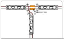
4. Modules may be connected in series or parrallel with connectors. Cap all unused wires. The strand of modules should not be looped to create a closed circuit.
