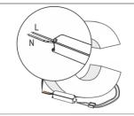
**8**. Finish by connecting AC power line to the input wires of the power supply.
