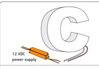
6. Run a wire from the power Supply to each channel letter and connect to the first LED module on the strip. Must be used with 12 V BaltLED Power Supplies.
